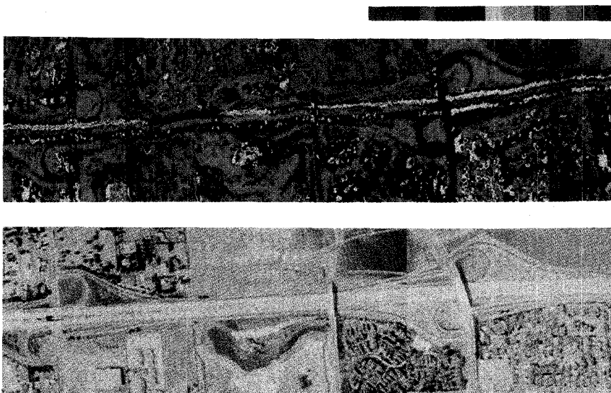
Fig. 8. Video and millimeter-wave images of a freeway scene near Simi Valley, CA, on Sept. 13, 1985. The 15-level color scale is from 250 K (dark blue) to 300 K (red). The scene width is 0.55 km with 173 data pixels across and the length is 2.1 km.
